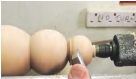
▲ Pic.4 Here the long point of the skew is used to cut the curve; this will require some practise, but it is incredibly satisfying once mastered
